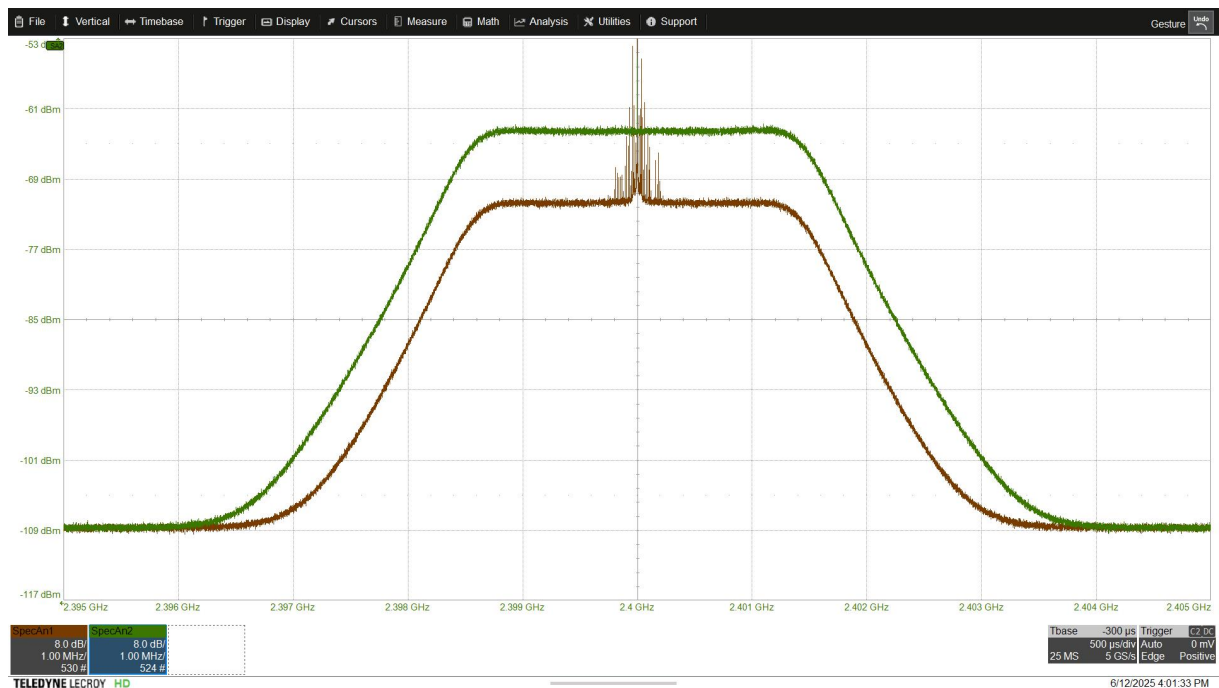
Figure 3.7: HackRF comparison: good performing device - HackRF 2 (green trace) and faulty device - HackRF 1 (orange trace) 1.75MHz filter response. Signal acquired with Lecroy WaveMaster 8330HD MSO.
