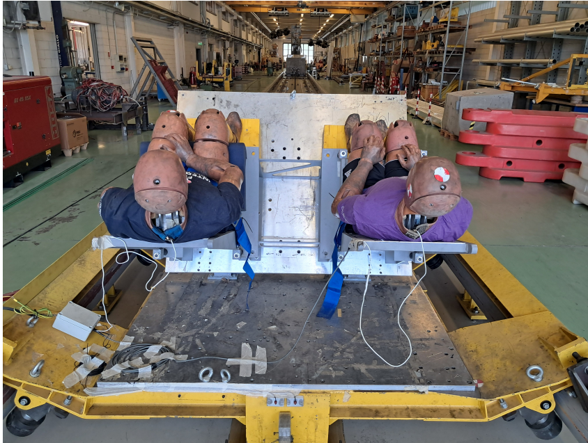
Figure 3.11: Instrumentation setup (Accelerometers and Load Cells)
