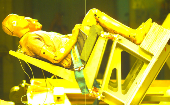
(c) K413, Frame 1171 – Maximum spring compression reached.
