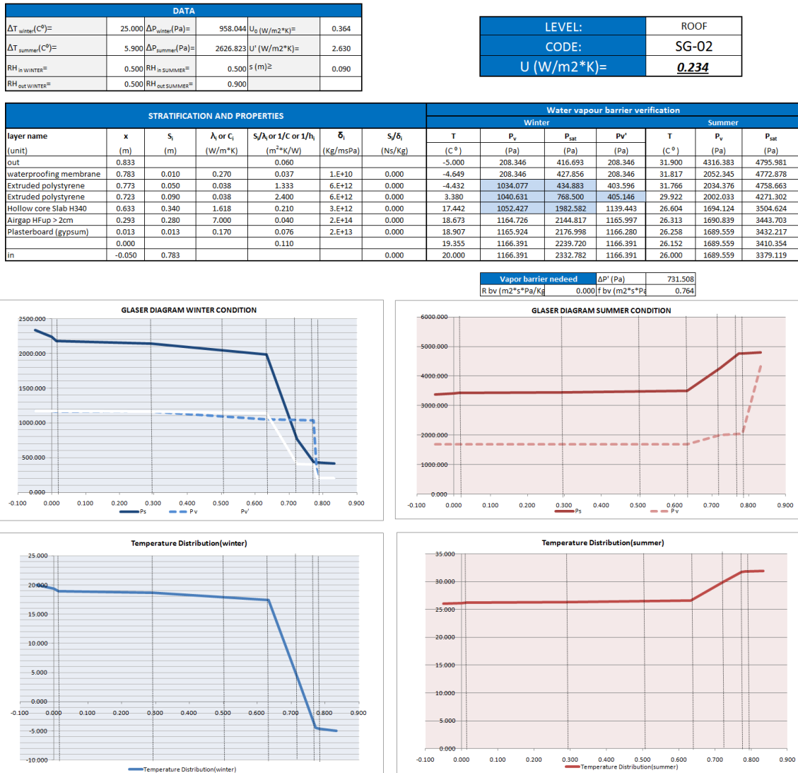
Illustration 145 Slab SG-02 Condensation risk analysis
