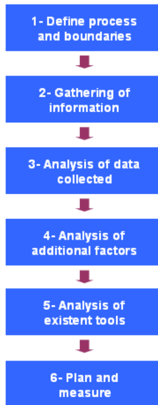
Figure 42: Steps for Implementing an Energy Consumption Monitoring System
