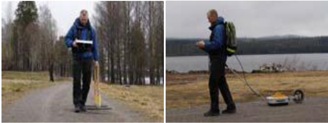
Figure 2.36: MALA ProEx GPR System in use to investigate the subsurface.
