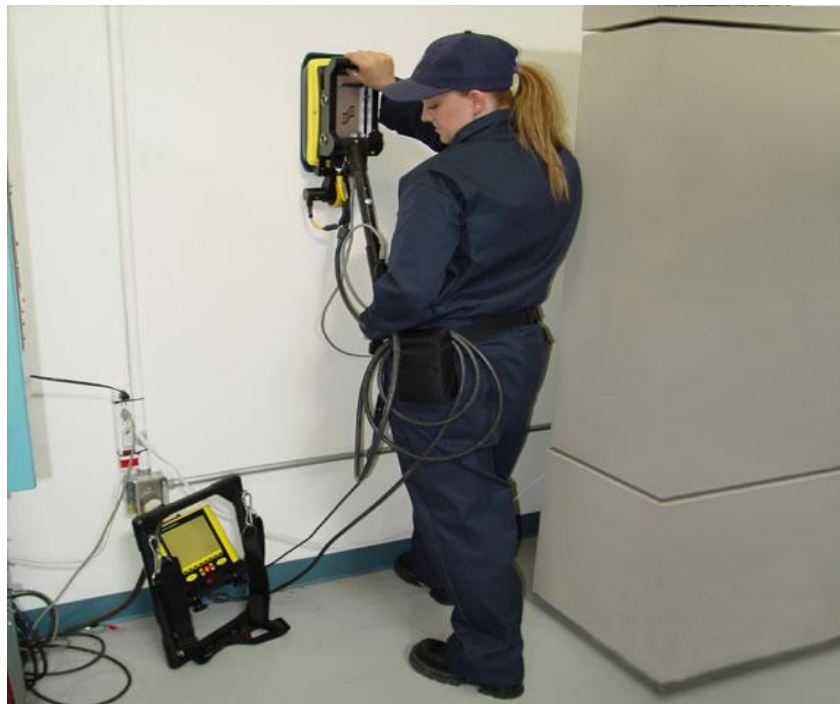
Figure 2. 19: SmartHandle GPR being used by a military for data acquisition.
