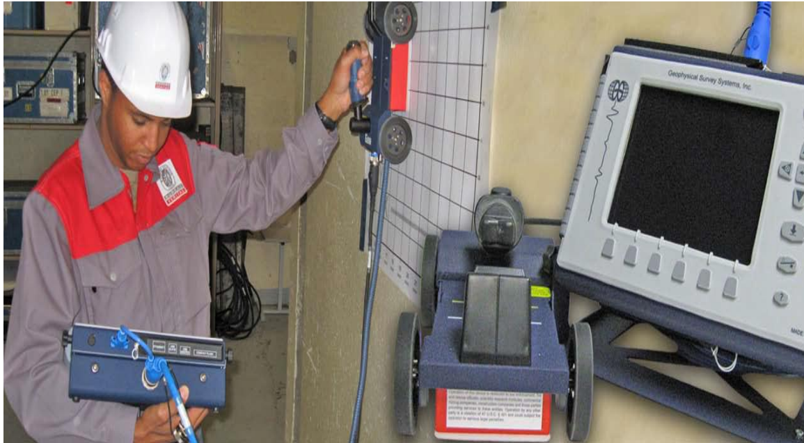
Figure 2.30: StructureScan Standard inspecting concrete wall.
