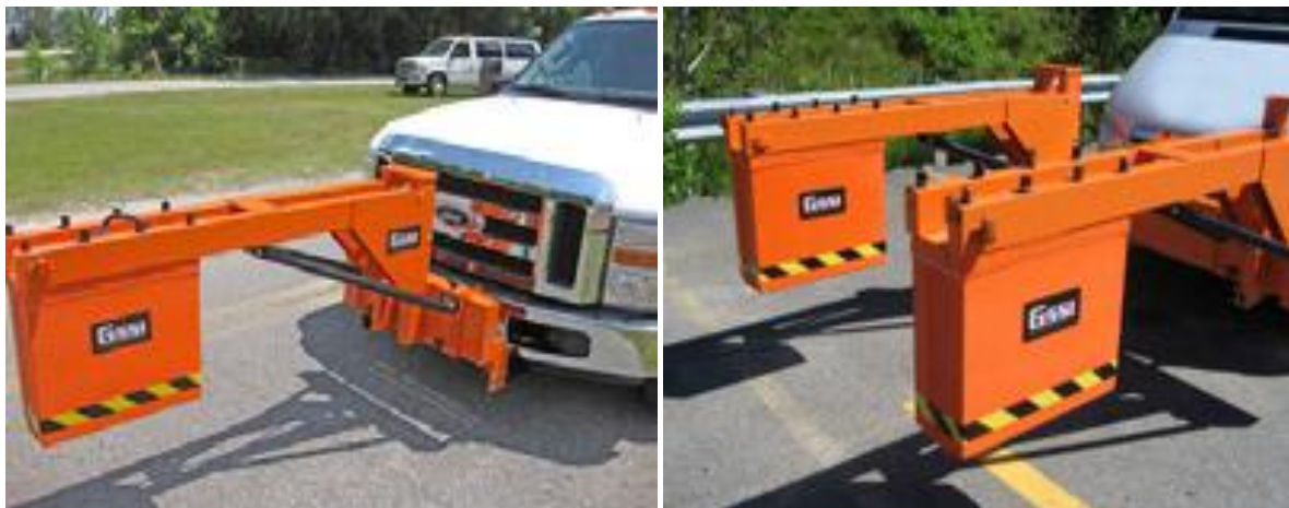
Figure 2.31: Single (left) and multiple (right) mount antennas RoadScan inspecting road.
