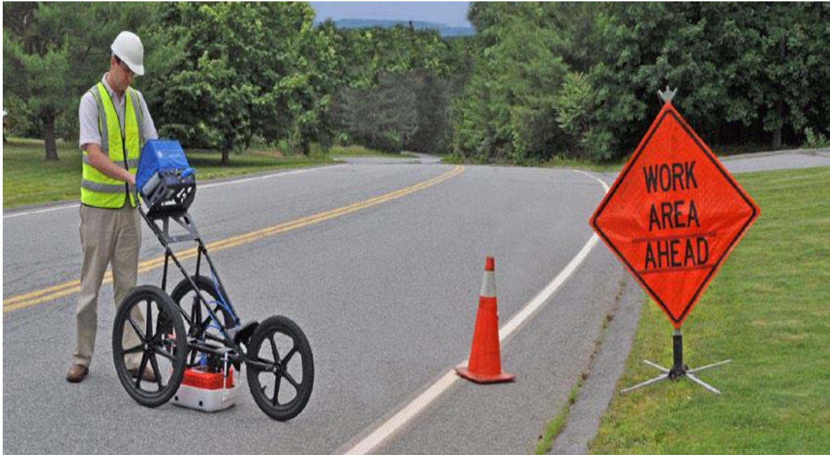
Figure 2.18: An operation making acquisition with a SmartCart GPR.
