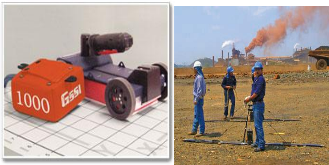
Figure 2.4: 1000MHz Deep Penetration Concrete Antenna on the left and Commercial GPR system with 25MHz Antennas on the right.
