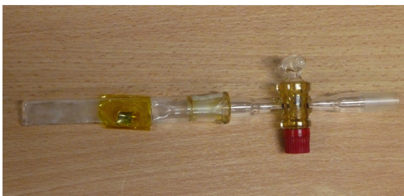
Figure 5.3: DEG sample inside the quartz cell that was keeping it under vacuum.
