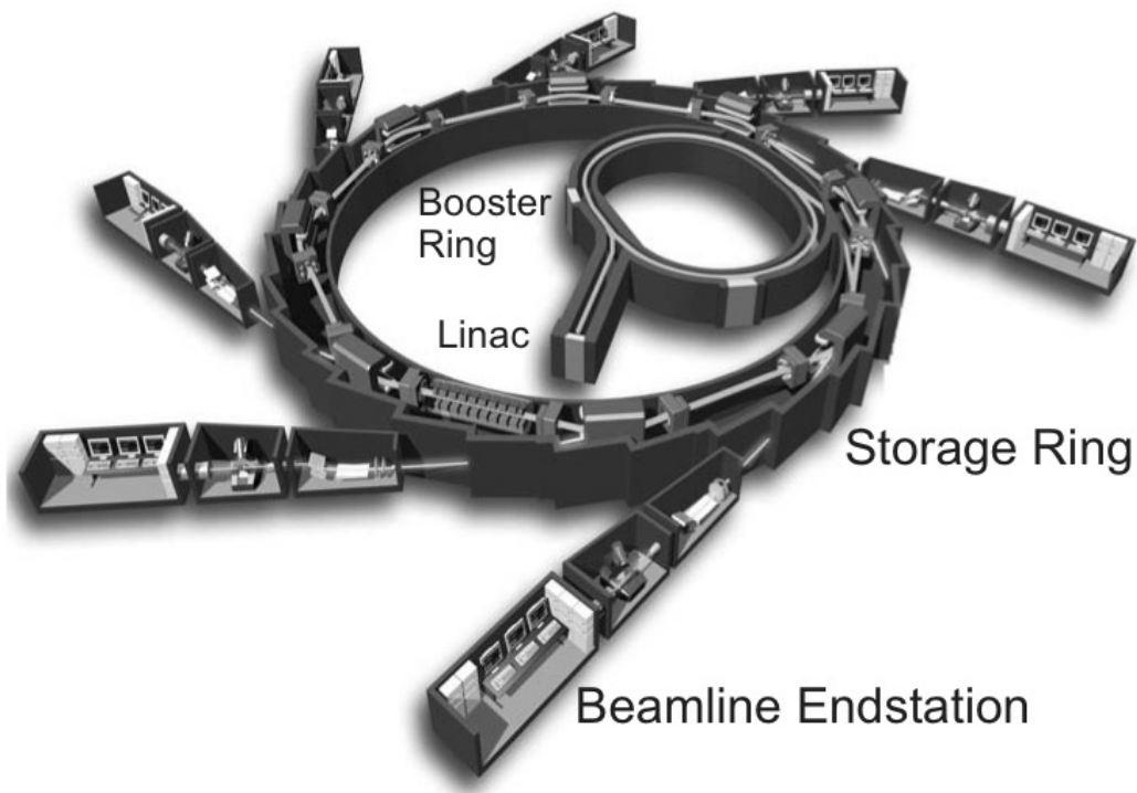
Figure 2.2: Typical schematic picture of a modern storage ring[44].
