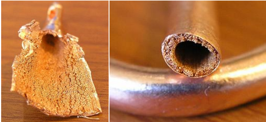
Figure 2.2 Sintered powder heat pipe (courtesy of Thermacore)
