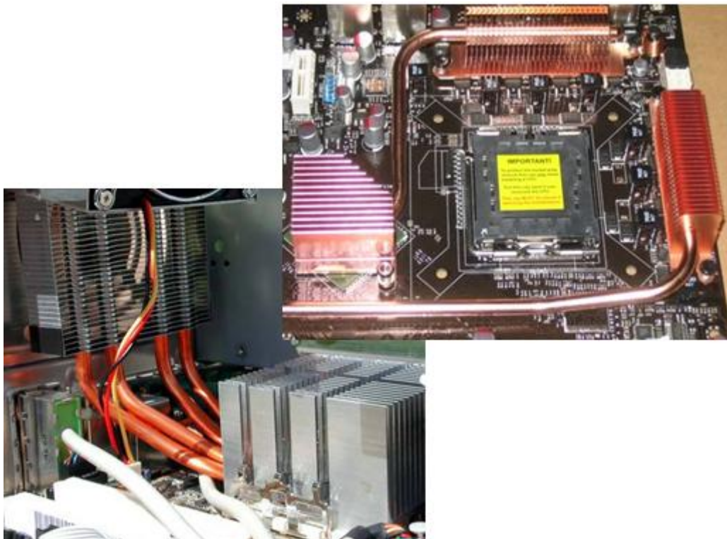
Figure 2.10 Heat pipes designed to direct the heat from the chipsets to the heat sink, where it can be carried away by airflow from a fan
