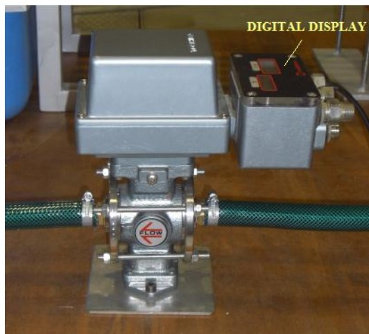
Figure 2.14. Detail of the electromagnetic flow meter.
