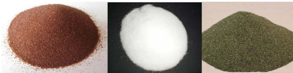
Figure 2.12: garnet (left), white alumina (middle), olivine (right)
