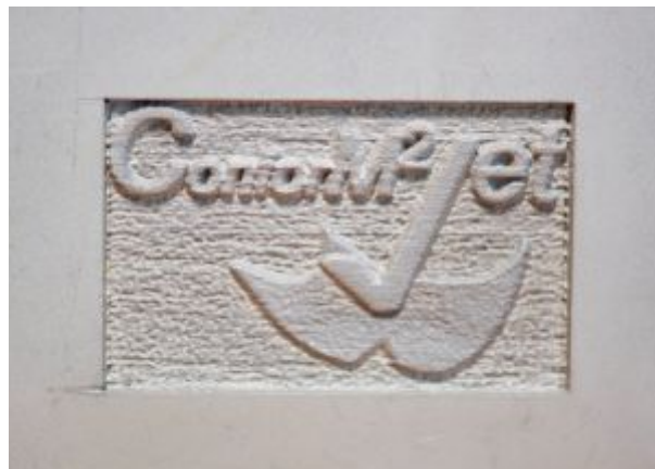
Figure 2.15: A shape obtained by water jet milling [32]
