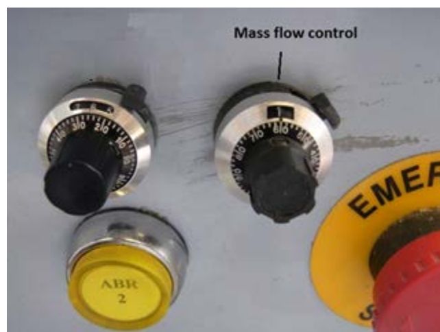
Figure 5.4: Abrasive mass flow control
