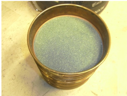
Figure 4.3: A load of abrasive (SiC)
