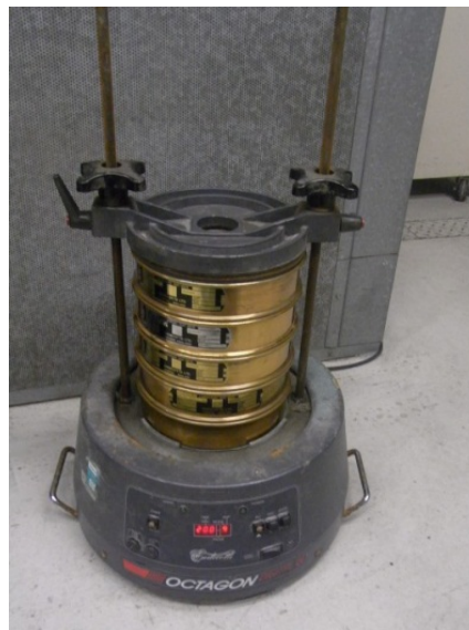
Figure 4.5: The sieving machine set up
