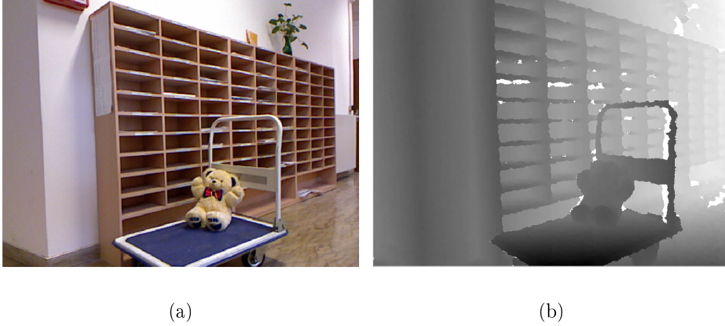
Figure 2.4: Examples of (a) an RGB image and (b) the corresponding depth map acquired with a Kinect.
