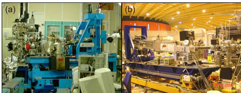
Fig. 2.6: Pictures of the AXES (a) and SAXES (b) spectrometers. AXES [21], installed at the ID08 beam line of the ESRF, is about 2.2 m long. SAXES [23] is a 5 m instrument, installed at the ADDRESS [20] beam line of the SLS.
