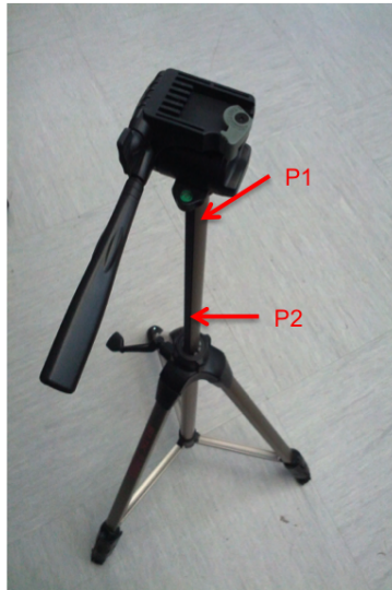
Figure 3.24: The photographic tripod used for vertical point intraoperative acquisition.
