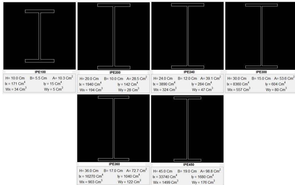
Fig.5. 22. Cross section areas of selected beams
