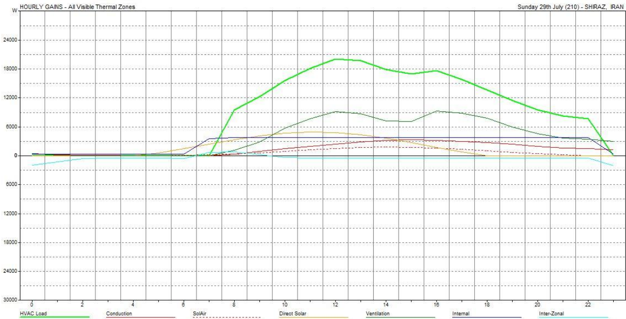
Fig.4. 64. Hottest Day Gains/Losses (Proposed Condition)
