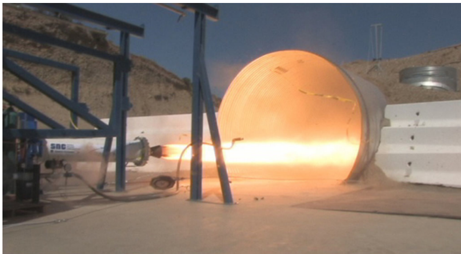
Figura 2.4: Sierra Nevada Corporation, Dream Chaeser Hybrid Rocket Motor Test
