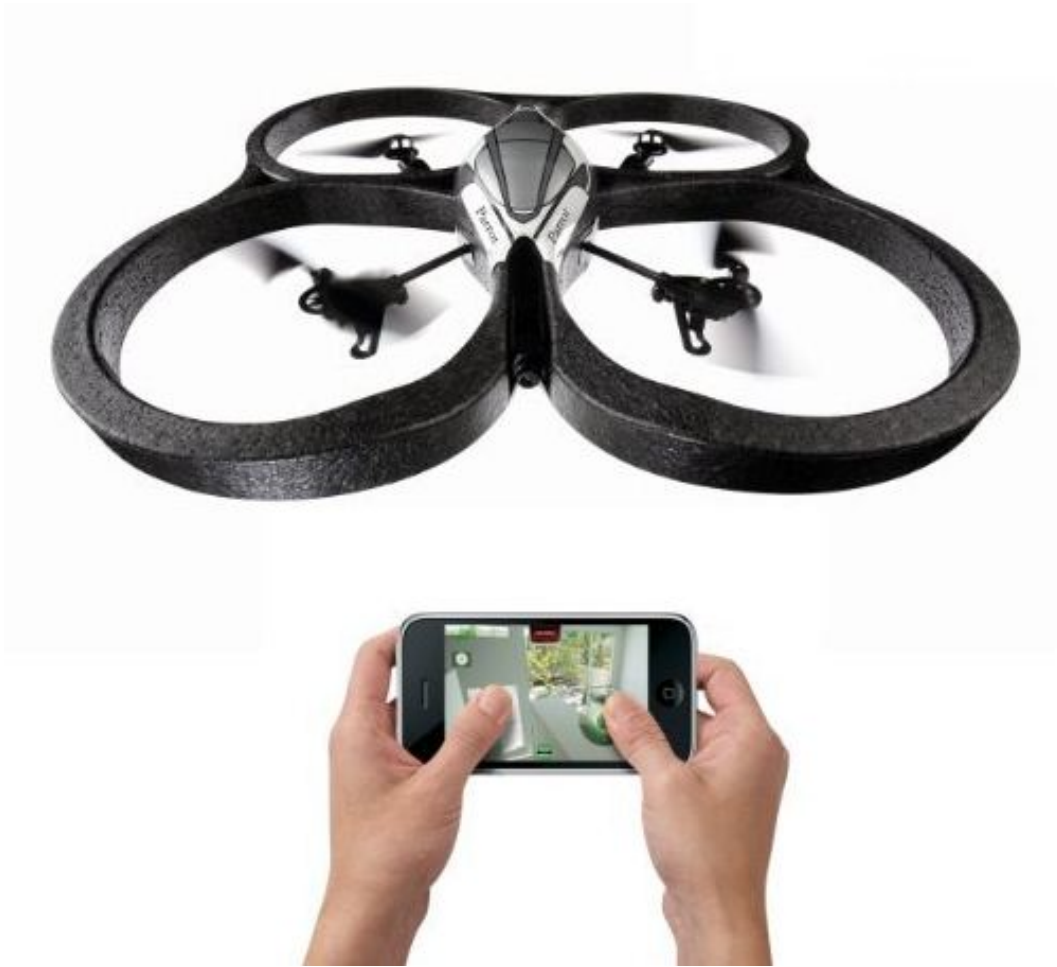
Figure 2: The Parrot AR.Drone, a commercial smartphone-controlled quadrotor.
