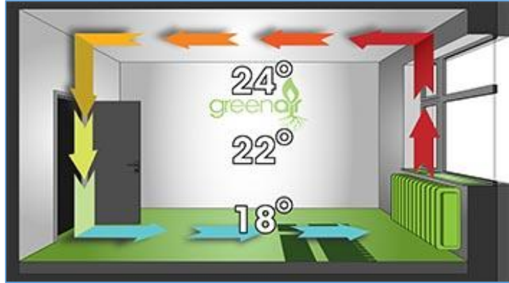
Figure 183 heat distribution by radiator
