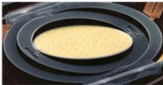
Figure 2.4 A stand alone two-axis micromirror for optical switching applications [73]
