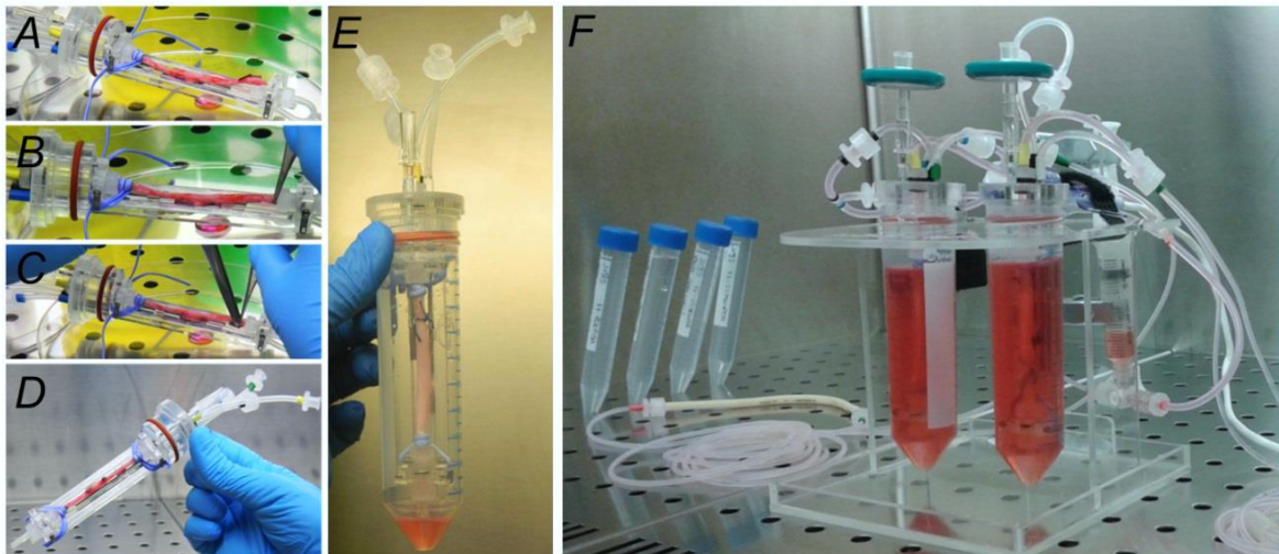
Figure 3.1. The compact and automated ex-vivo vessel culture system able to artificially produce the effects of the pulsatile arterial pressure-related cyclic wall distention. The EVCS during system assembling under laminar flow hood: the SV segments are cannulated on both ends with barbed luer fittings, and bounded on the connectors using a vessel loop (A-D). Then, the SV housing is inserted within the 50-ml falcon tube acting as reservoir (E). Once assembled, the culture chamber is connected to the stimulation circuit (F).
