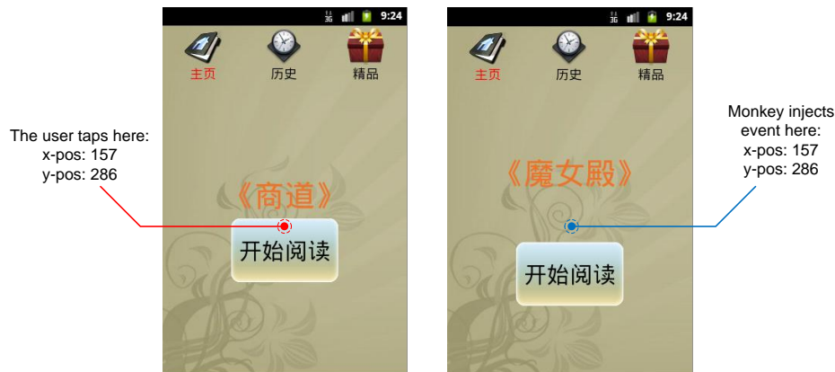
Figure 3.12: Failure example of a monkey-based test re-run.
