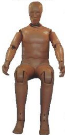
The FAA Hybrid III 50<sup>th</sup> Percentile Male ATD is a dummy produced under a cooperative between the Federal Aviation Administration (FAA), Civil AeroMedical Institute (CAMI), Denton ATD, Inc., and Robert A. Denton, Inc., for the sole purpose of Federal Aviation seat certifications.
