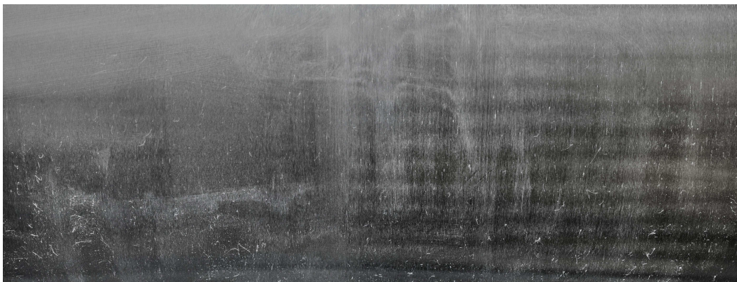
Figure 3.7: Example of a cylinder presenting chatter marks only on the right side.
