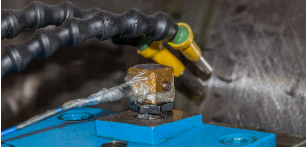
Figure 3.1: A detail of one of the accelerometers placed on the machine.
