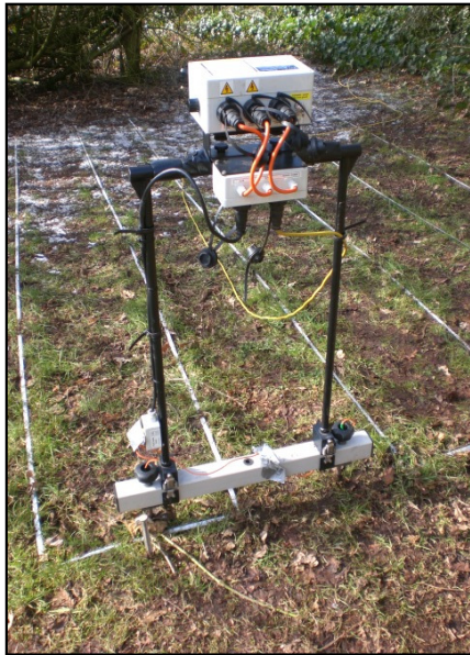
Figure 3.1: Custom built frame used for constant offset resistivity survey
