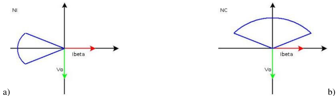
Figure 7-37: Intervention sectors definition in blue, a) for isolated network (NI) and (b) for compensated network (NC)
