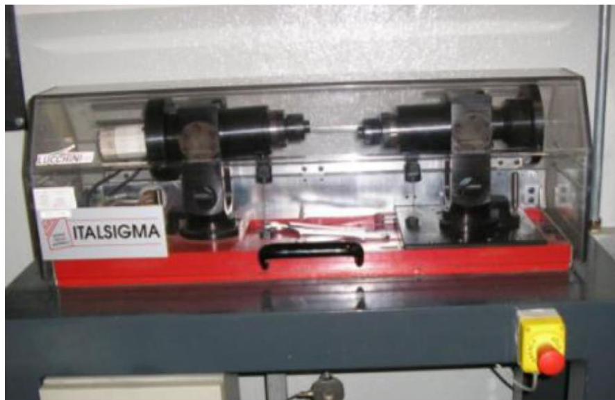
Figure 4-8. Rotating bending fatigue test machine used in the present work.
