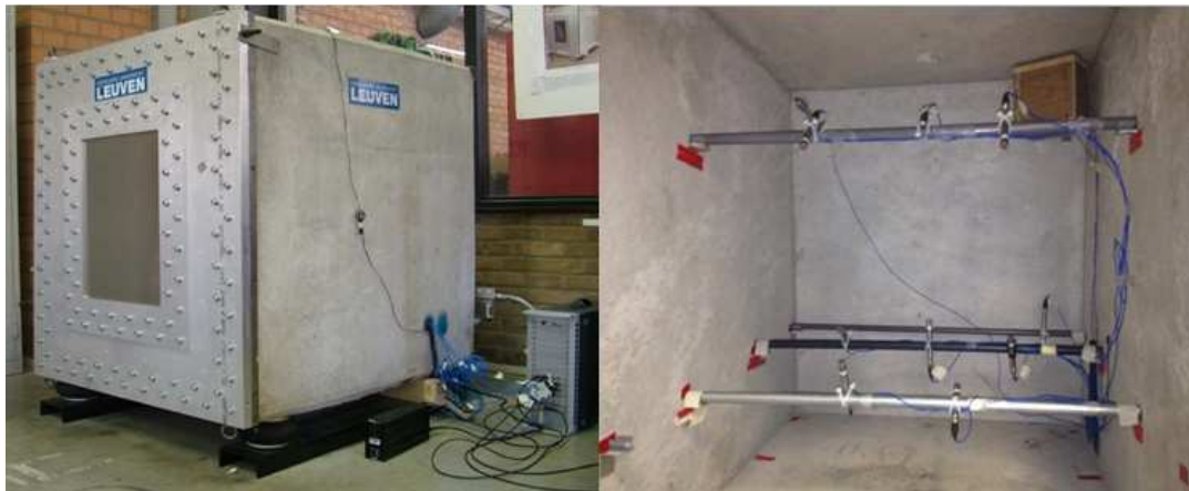
Figure 99 - PMA Sound Box: exterior (left), interior (right).
