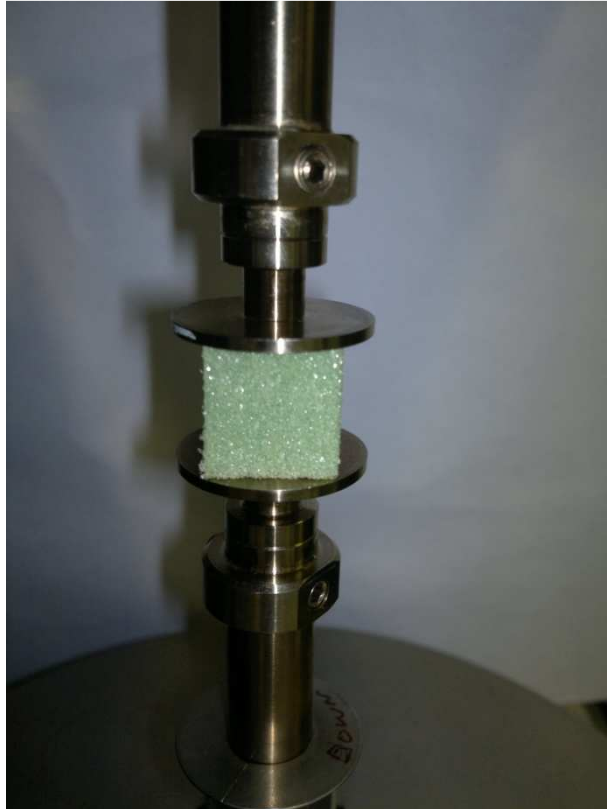
Figure 67- Clamped foam specimen.
