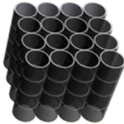
Figure 27 - Porous material as assembly of parallel tubes.
