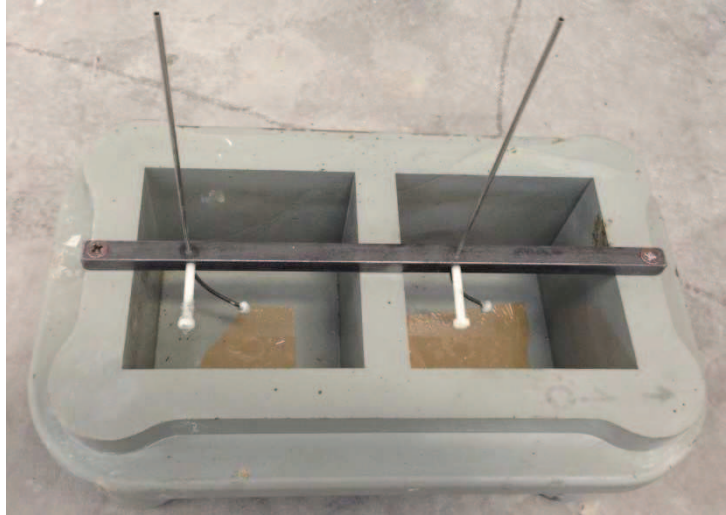
Figure 84: Cubic molds for pore pressure specimens, instrumented with curved pipes.
