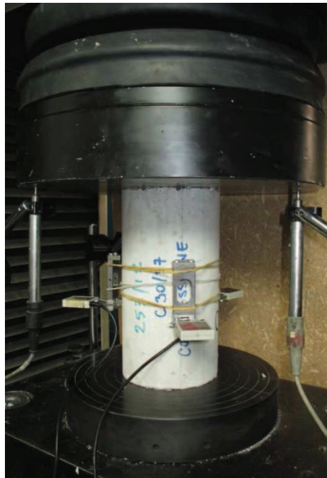
Figure 81: Instrumented specimen tested in compression (controlled displacement).
