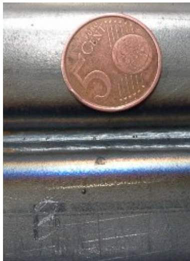
Figure 7-66 CMT welding, V=20 mm/s
