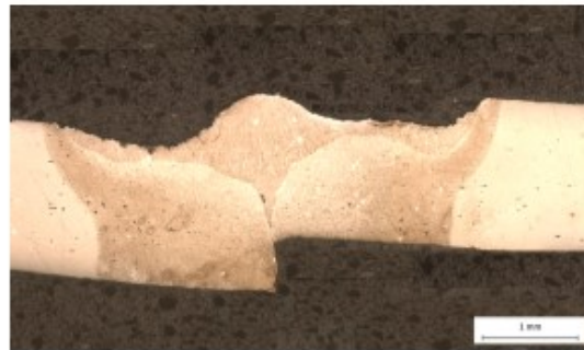
Butt joint, V=30 mm/s
