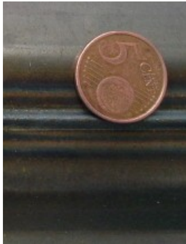
Figure 7-63 CMT welding, V=20 mm/s
