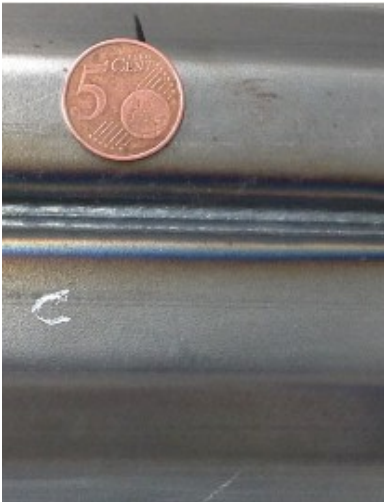
Figure 7-73CMT welding, V=22 mm/s
