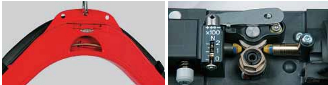
a. The new tension-lever system in the welding torch ensures constant and reproducible contact pressure. b. The wire buffer decouples the front and rear wire-drives from one another and ensures smooth wire travel.
