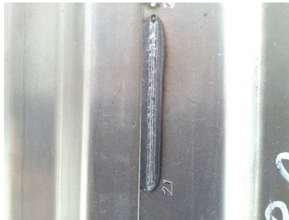
Figure 7-46 P=3 Kw, V= 30 mm/s
