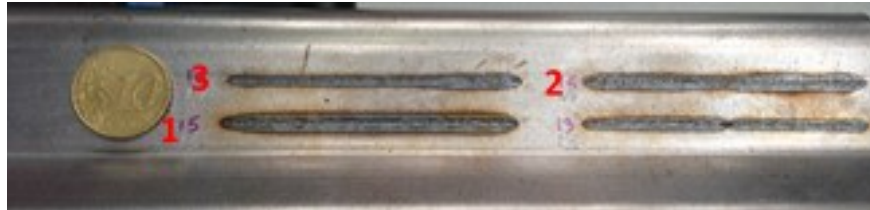
Figure 7-37 Welding on bop configuration, P=3Kw, V= 30 mm/s
