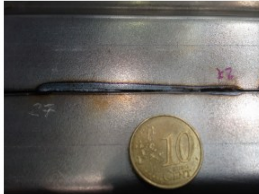
Butt joint, P=3Kw, V=30 mm/s
