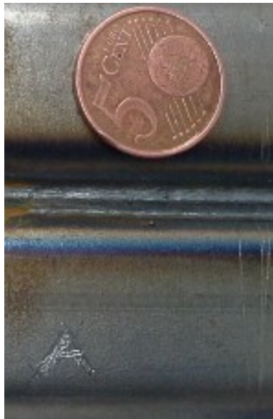
Figure 7-68 CMT welding, V=25 mm/s
