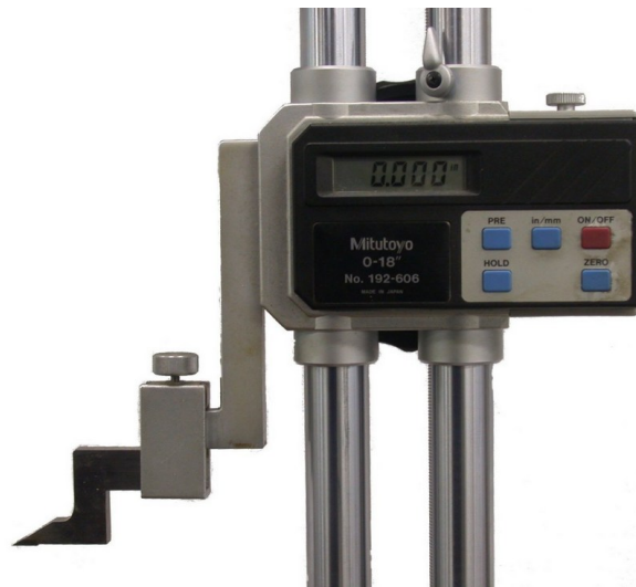
Figure 7-33 Height gauge used for measuring planarity of pipes
