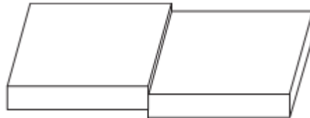
Figure 2-7 Welds made on mismatched joints often will fail below the rated load when placed in stress conditions
