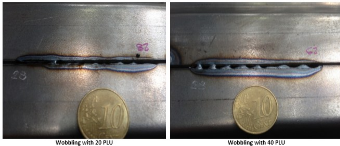
Figure 7-49 Butt joint, P=3Kw, V=30 mm/s
