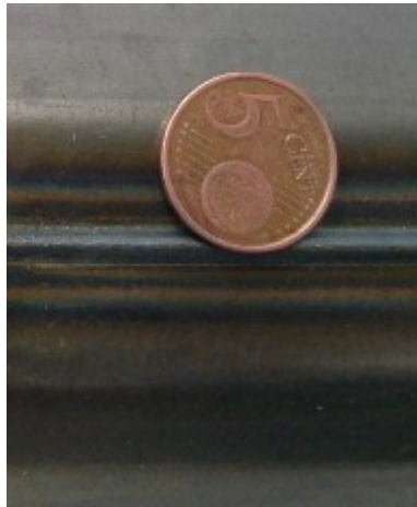
Figure 7-70 CMT welding, V=17 mm/s
