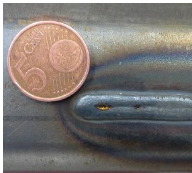
Figure 7-58 CMT welding V=10 mm/s
