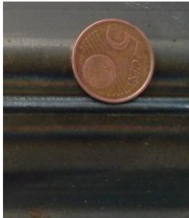
Figure 7-60 CMT welding, V=20 mm/s
