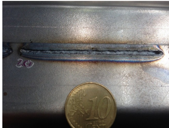
Figure 7-43, P=3 Kw, V=30 mm/s, Wobbling 20 PLU
