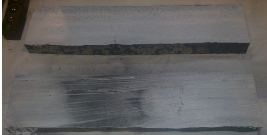
Figure 65: The two samples for magnetic particle testing
