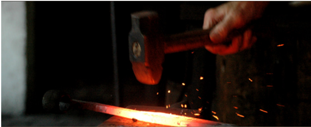
Figure 9: Hammering of wrought iron
