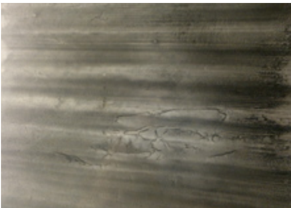
Figure 66: Cracks identified with magnetic particle test
