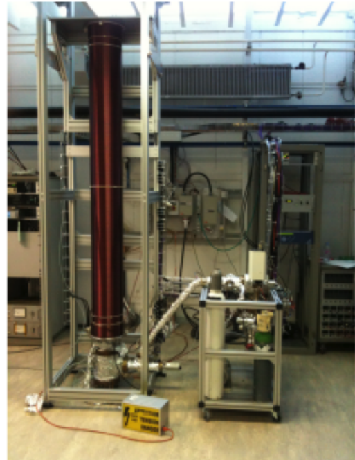
(b) Deposition system during the coating when the magnet is lower over the tower.
