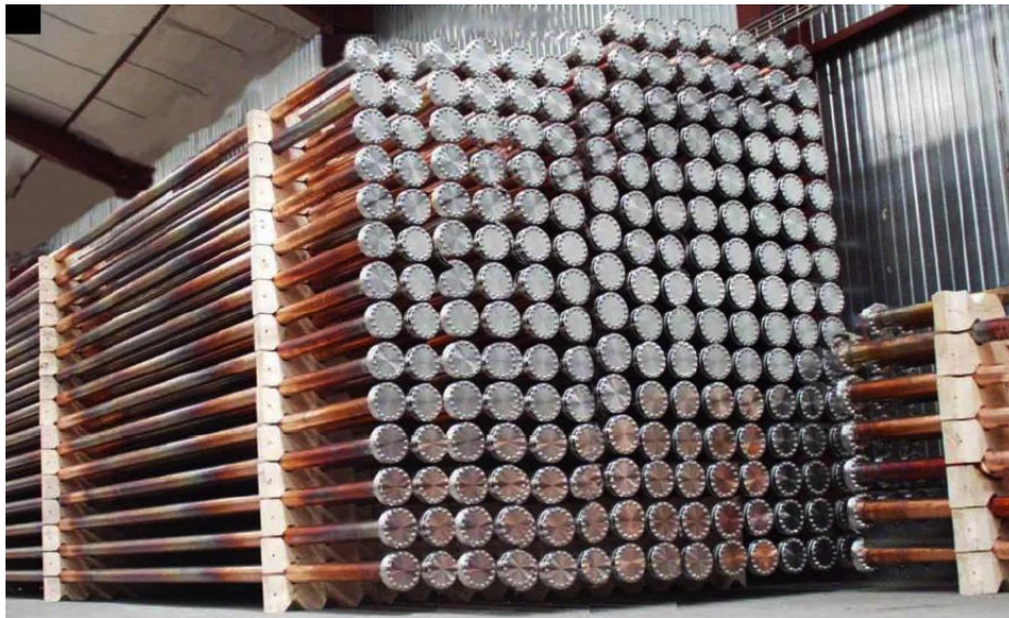
FIGURE 1.7: A stock of NEG coated vacuum chamber ready to be installed in the LHC tunnel.
