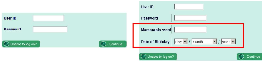
Figure 2.4: Example of a real injection on the login form in a web page of online-offshore.lloydstsb.com .
