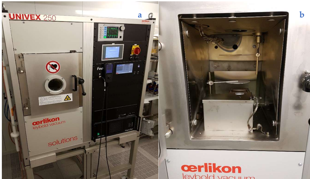
Figure A.3 (a): Electron beam evaporator
