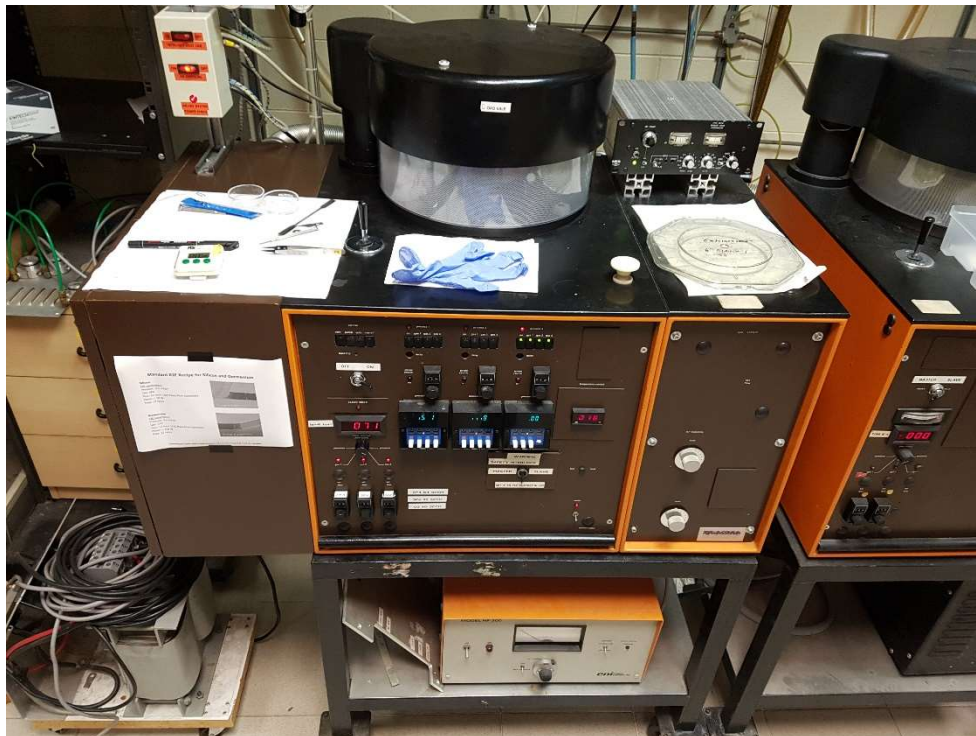
Figure A.4: Parallel-plate Reactive Ion Etcher. On top the vacuum chamber can be seen. On the bottom, all experimental parameters (gas flux, chamber pressure, Plasma power...) can be adjusted.
