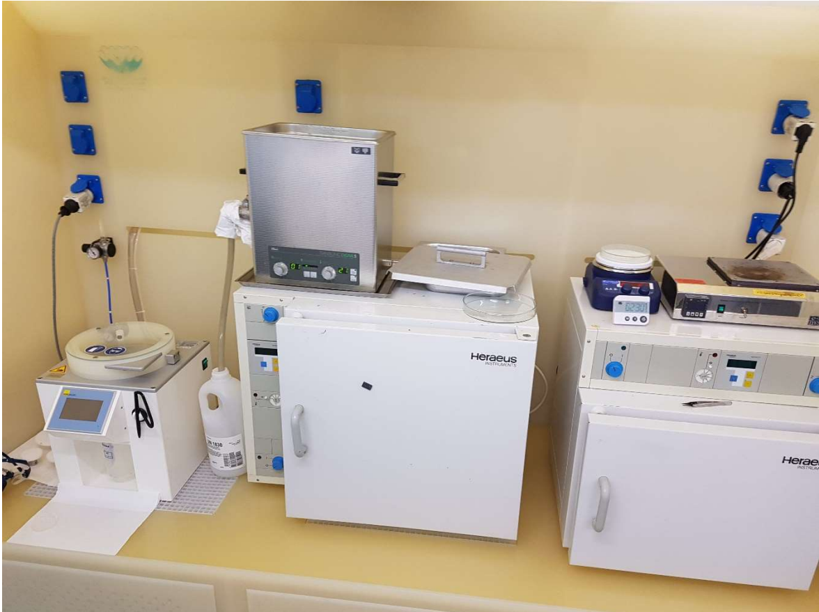
Figure A.1: Working station with spin coater and hot plates, in clean room ambient, where polymers are coated and spun and where bakings occur.
