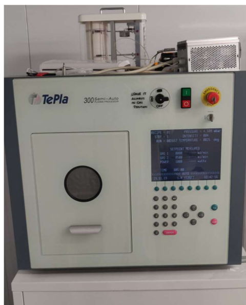
Figure A.5: Plasma asher chamber on the left. Monitor to keep under control experimental parameters on the right.
