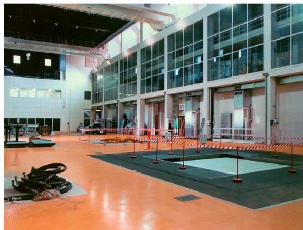
Figure 95 : Shaking table, 4m x 4m, of the Research center ENEA Casaccia (Rome).
