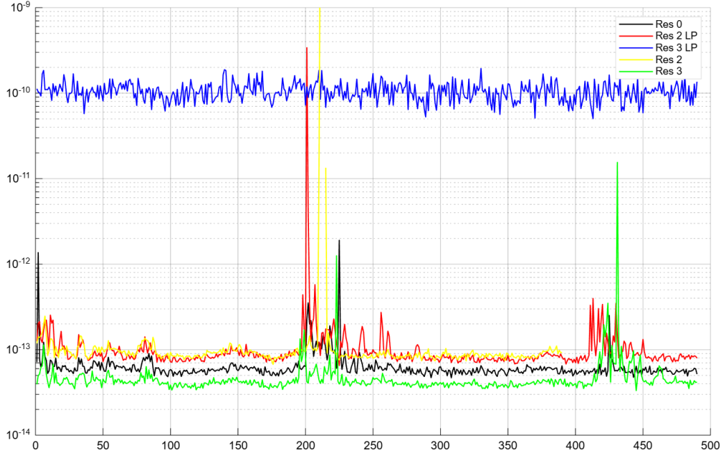
Figure 4.1: Comparison of residual norms over the first 500 time steps for the different solvers.
