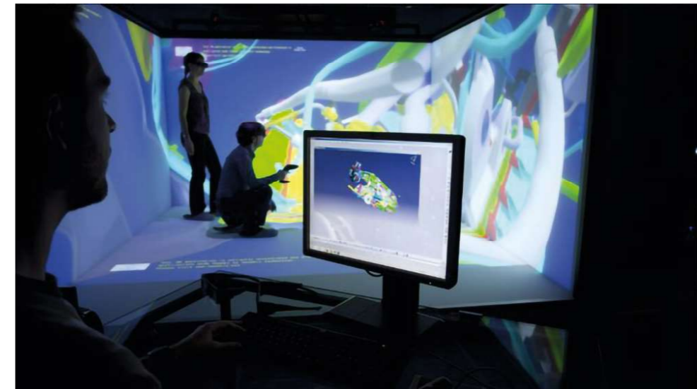
Figura 2.11: Dispositivo Cave. Fonte: Muhanna, M. A. Virtual reality and the CAVE: Taxonomy, interaction challenges and research directions. J. King Saud Univ. - Comput. Inf. Sci. 27, 344-361 (2015)
