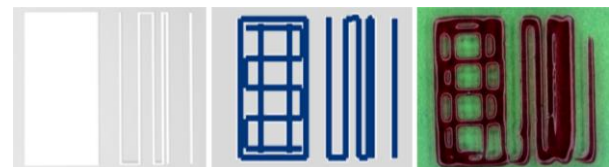
Figure 2: The input model from the design (left) to the g-code (center), to the final print picture (right).
