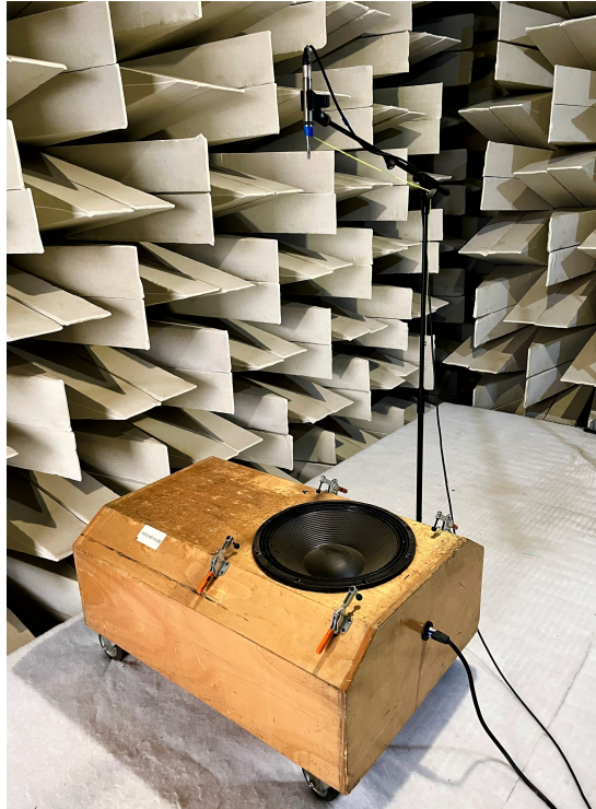
Figure 3.1: SPL measurement in anechoic room with a free-field pressure microphone. The loudspeaker is placed in a closed box that is an approximation of the infinite rigid baffle where acoustic short circuit is not present. As explained in section 2.3, Rayleigh total SPL computation refers to an infinite baffle response where acoustic short circuit is not taken into account. Not being the box infinitely extended, some deviation between the measured and calculated SPL is expected.
