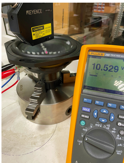
Figure 3.2: Amplifier output RMS voltage measurement with a Fluke 289 multimeter.
