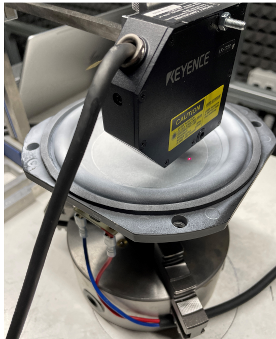
Figure 3.3: Loudspeaker cone treated with white 3D scanning powder.
