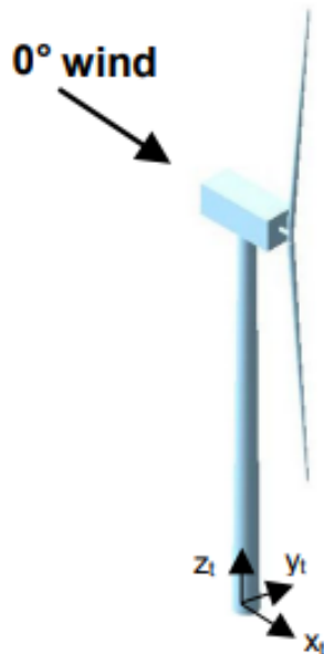
Figure 3.7: Tower top coordinates reference system. It is fixed to the support platform, so it rotates and translates with the platform. x_t points the nominal downwind direction.
