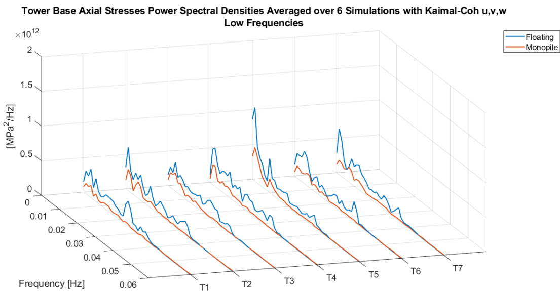
Figure 5.8: Tower base axial stresses power spectral density for each wind turbine and for both floating and monopile case, in the low-frequency range with Kaimal-Coh u, v, w turbulence.
