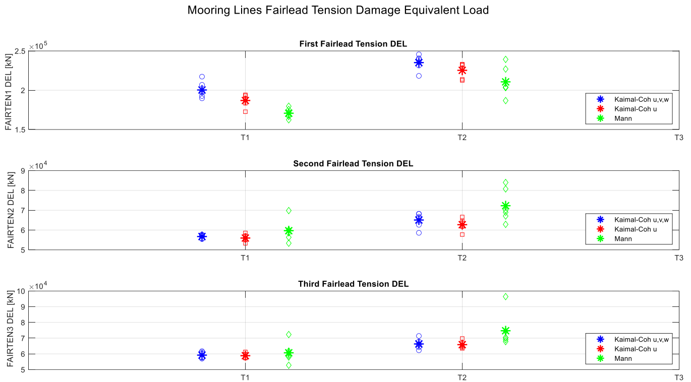
Figure 3.21: Mooring lines short-term DELs for each wind turbine and turbulence case. Each marker represents the mean value of one simulation except for the asterisk, which represents the average over the six simulation.
