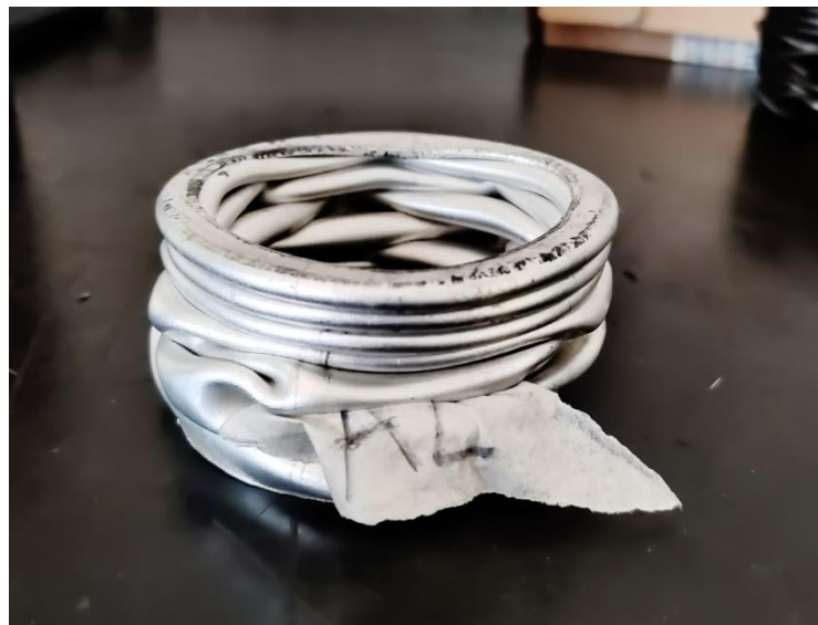
Figure A.5: AL tube after impact.
