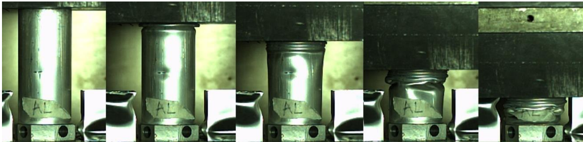
Figure 3.8: AL tube crushing dynamic.
