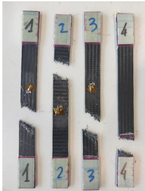
Figure A.3: Failure mode of in-plane shear test specimens.
