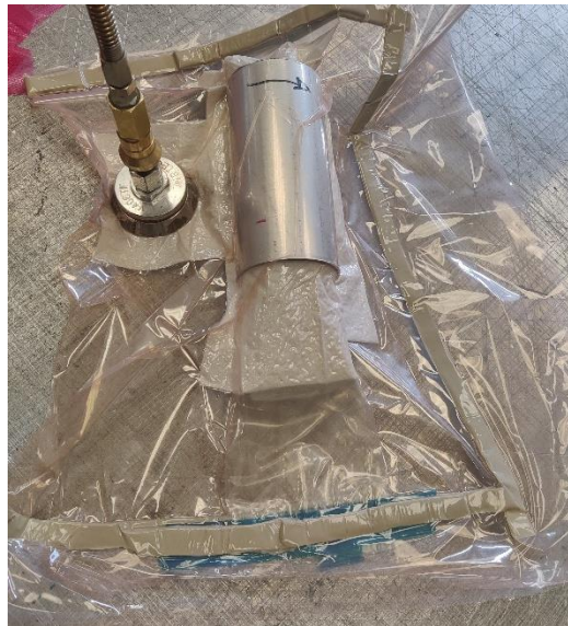
Figure 2.7: Reusable vacuum bag for mid-lamination compaction
