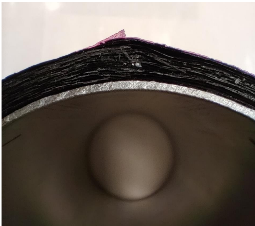
Figure A.1: Detail at overlapping point in external lamination.
