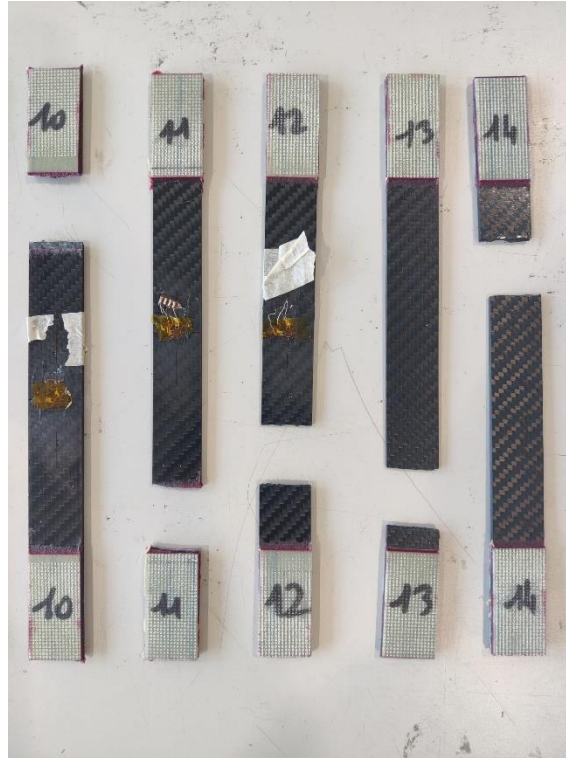
Figure A.2: Failure mode of tensile test specimens.
