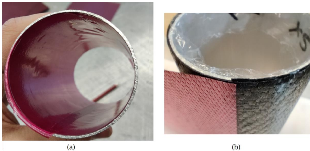
Figure 2.5: Close up picture of (a) internal application of structural adhesive, (b) the overlapping spot for external lamination.
