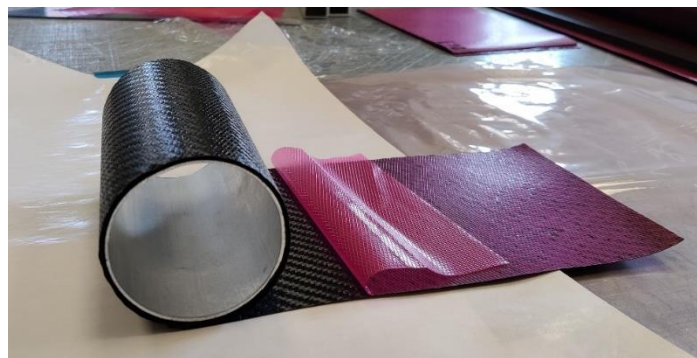
Figure 2.4: Cut prepregs during the lamination.
