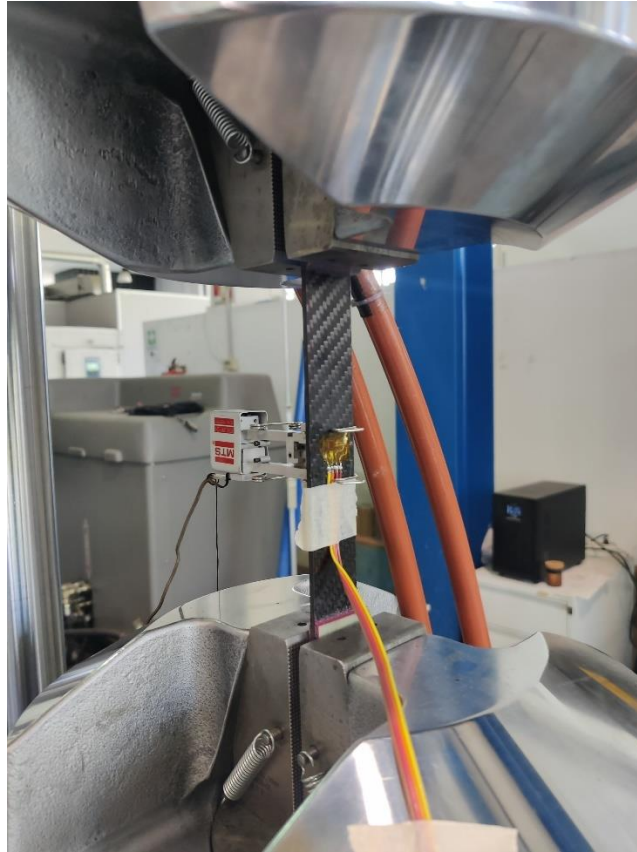
Figure 3.2: Tensile system setup.
