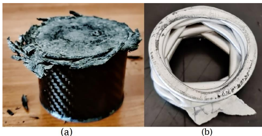
Figure 0.1: Circular tubes after impact (a) composite, (b) ductile.
