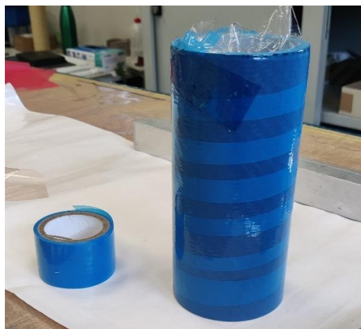
Figure 2.6: Heat-shrink-tape applied during lamination process.
