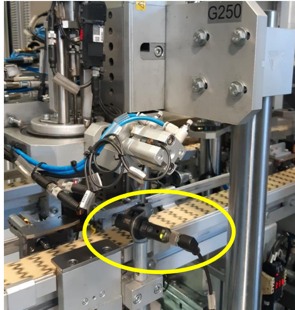
Figure 3.8 Proximity sensor as a stopper to limit buffer capacity
