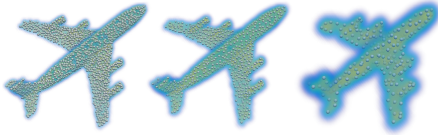
Figure 4.1: Image from [2] explaining how the extension operator works: the image is showing three Point Clouds (composed of 2048, 1024 and 256 points respectively) where each point is associated to a single, unitary feature. The colored area represent the continuous, d -Dimensional (here d = 3 ) function returned by the extension operator for each of the three Point Clouds. It is possible to note how the shape of said function is independent with respect to the cardinality of the Point Cloud that was used to generate it.
