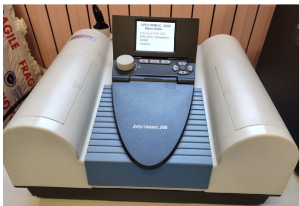
Figure 2.11: Image of the spectrophotometer SPECTRONIC 200E.
