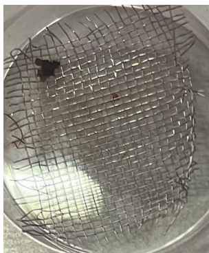
Figure 2.9: Image of thin titanium net where free-standing membranes were deposited.
