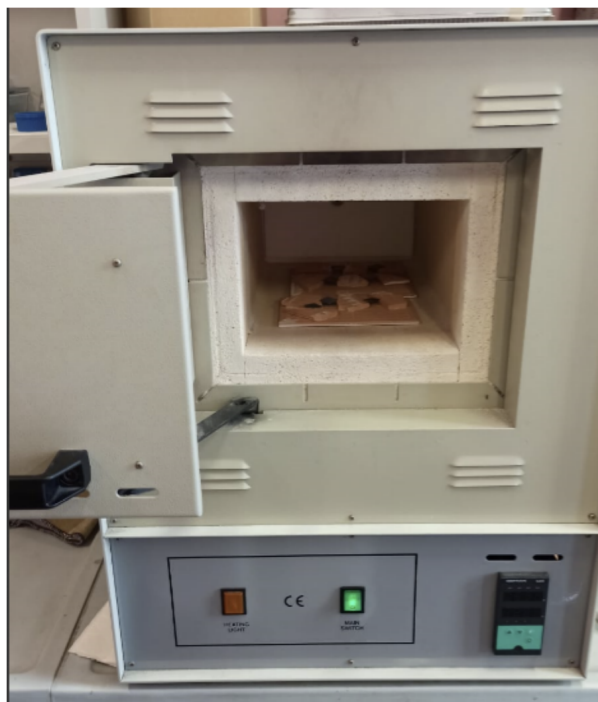
Figure 2.6: Frontal view of a GEFTRAN 1200 oven and its inner room surrounded by ceramic porous walls.
