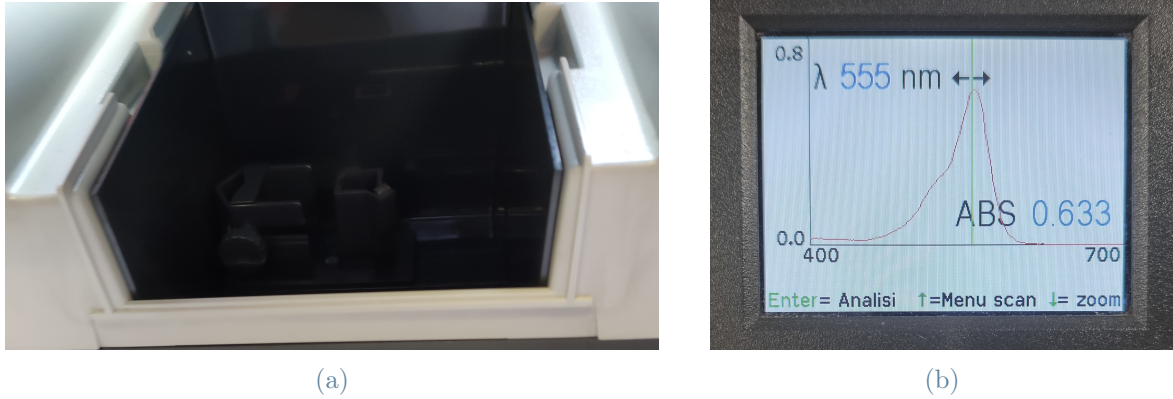
Figure 2.12: (a) Image of the cuvette holder inside the spectrophotometer. (b) Example of absorbance spectrum exhibited on the display of the spectrophotometer.
