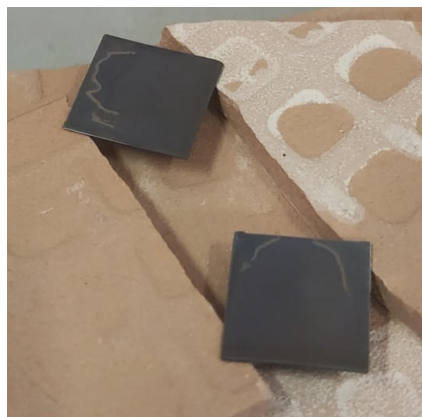
Figure 3.7: Close-up image of two 2 cm X 2 cm samples before annealing, exhibiting pale yellowish lines that map the compromised area after the second anodization.
