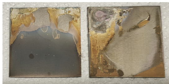
Figure 3.12: Close-up image of the two samples obtained from the mixture of two nearly exhausted electrolytes, highlighting the defects originating from dielectric breakdown phenomena.
