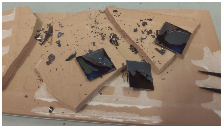
Figure 3.2: Visual representation of the condition of three fragile TiO_2 layers after annealing. Surrounded by small fragments and debris, the remaining films appear curled up due to the different thermal stresses of the oxide layer compared to the metallic substrate.
