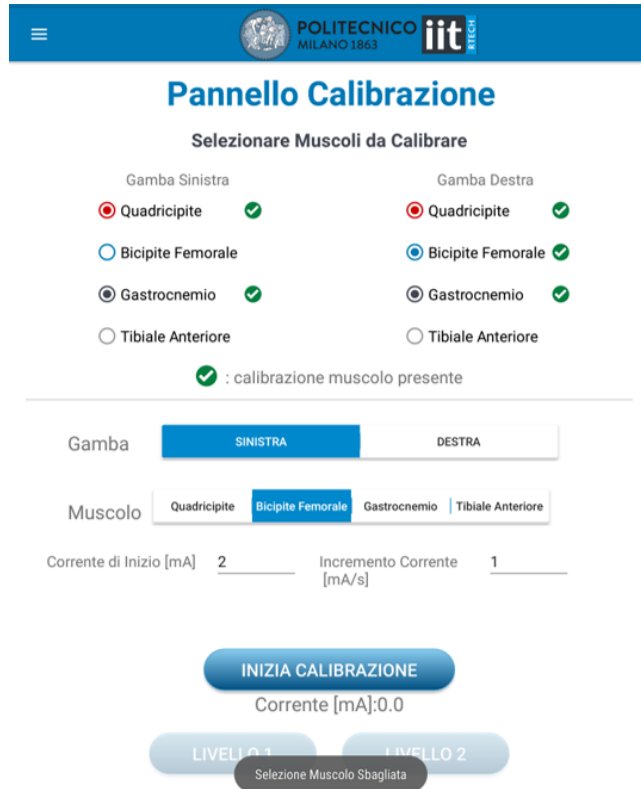
Figure 7: Advice of wrong muscle selection and visualization of muscles that are already calibrated.
