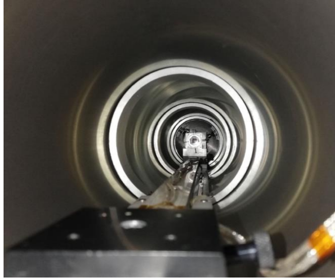
Figure 2.13: image of the interferometer from the end of the chamber. The second grating is clearly visible.
