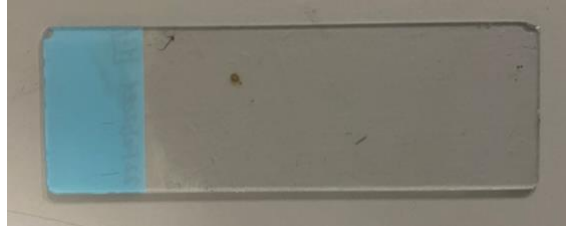
Figure 2.27: image of the glass support used to deposit the emulsion
