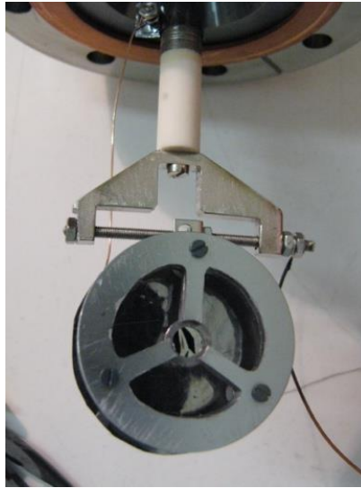
Figure 2.5: image of the moderator and its support, ready for the thermal treatment.
