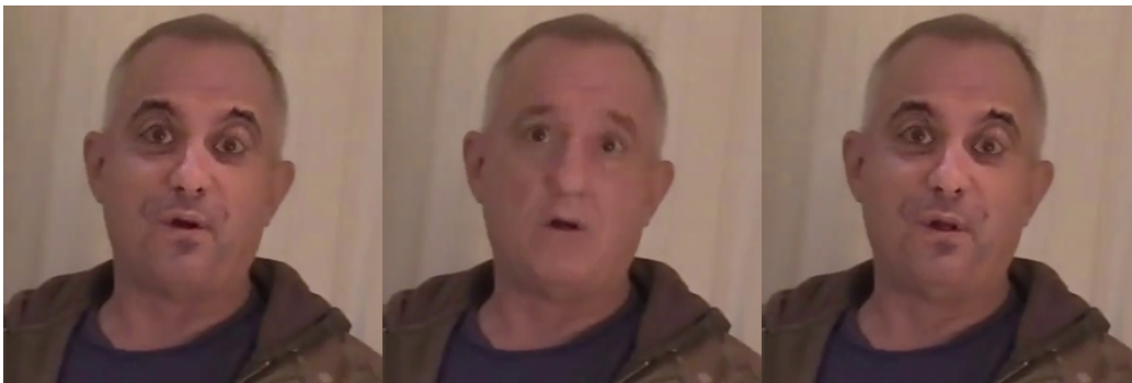
Figure 5.13: Example of the flickering effect in three consecutive frames. Here the effect is pretty strong and noticeable, even frame-by-frame. In the middle frame we can see how the deepfake generator has failed in detecting the face and therefore in generating the modified face for that frame. Sample taken from the DFDC dataset.
