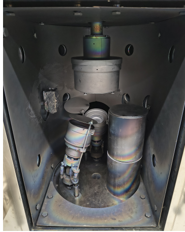
Figure 5.2: Image of the components inside the vacuum chamber of the HiPIMS setup.
