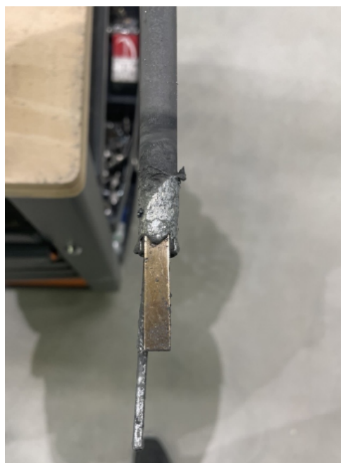
Figure 7.2: Photo of a sample after exposure. Residual solidified Pb is covering the screw connecting the sample to the shaft.
