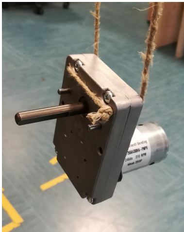
Figure 2.2: Model 2 gearmotor suspended for testing
