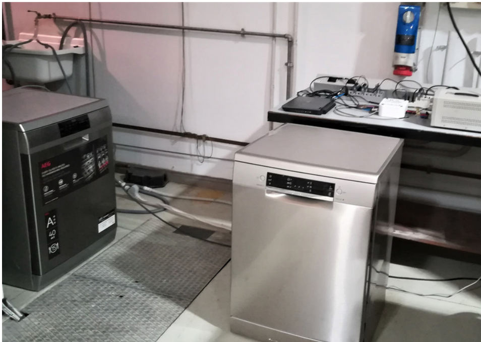
Figure 2.5: Experimental setup to measure dishwashers current and voltage
