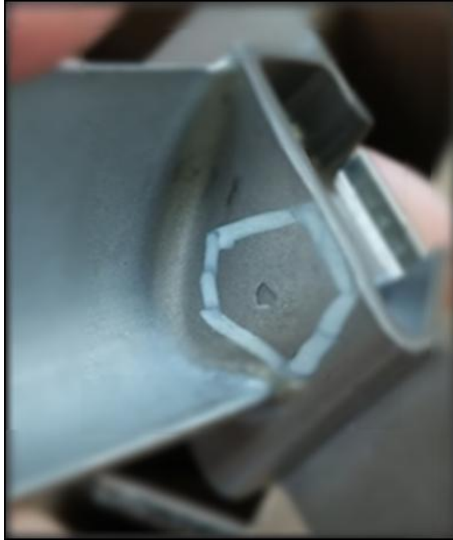
Figure 13. Inclusion at the surface of a blade root [36]
