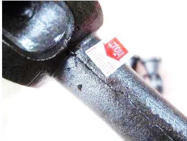
Figure 20. Example of a hot crack in the surface of the sample
