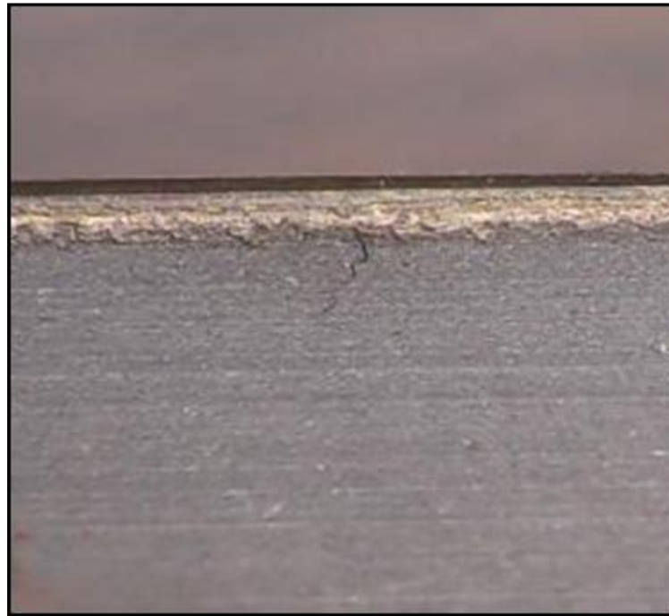
Figure 18. Example of a 3mm surface crack [37]
