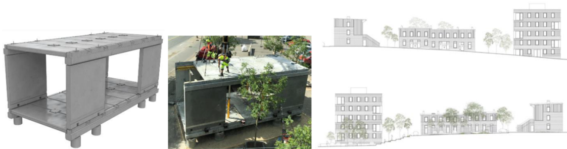
Figure 24: concrete building blocks structure of the Circle House
