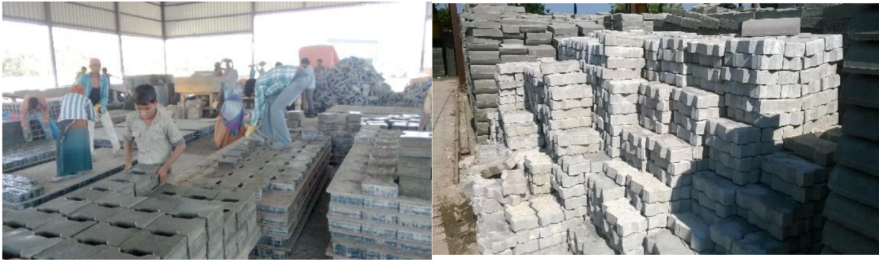
Figure 25: finished product made of processed wastes
