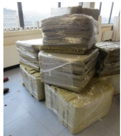
Figure 21: Horta-ONSS materials ready to be reuse off-site
