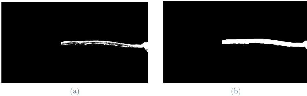
Figure 4.10: (a) Result of cv2.inrange function. (b) Result after the dilation transformation.
