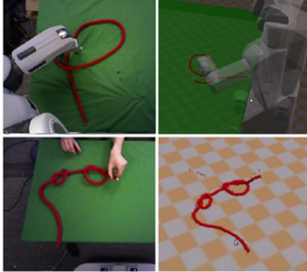
Figure 2.10: Example of DLO tracking using the GMM-EM with a physics simulator [6].
