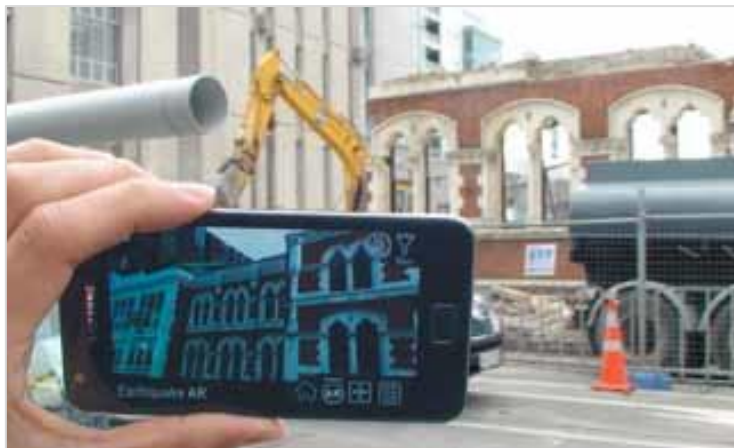
Figure 9 - CityViewAR showing virtual building on-site in AR view [80]
